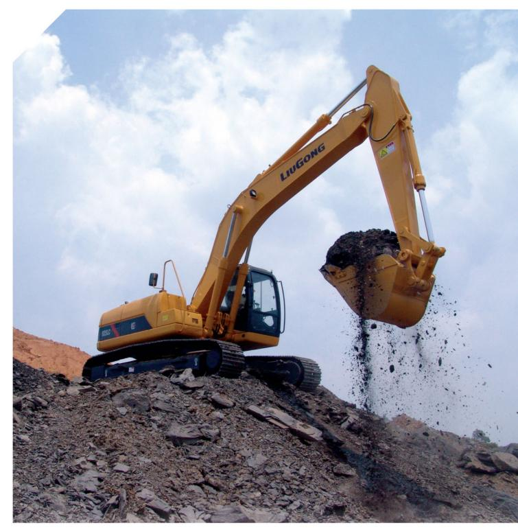
**Bucket Capacity** 0.73-1.2m<sup>3</sup> **Rated Power** 125kW/2100r/min **Net Power** 115kW/2100r/min Operating Weight 22500kg
