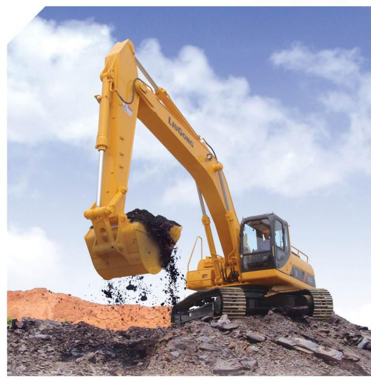
**Bucket Capacity** 0.73-1.05m<sup>3</sup> **Rated Power** 108kW/2100r/min **Net Power** 98kW/2100r/min Operating Weight 21900kg
