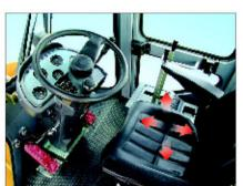
Adopt new type noise and shock absorbers to absorb to the most extend. Just 85dbs nearby drivers' ear. Arosal absorption of shock professional seat can be adjusted in all direction, satisfied various taste. Equipped with electrical fuel gauge and preserved dip-stick for oil-checking convenience.
