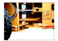
Extended distance of articulated points gives enlarged room for maintenance. Transmission shaft is designed above the lower linkage point to prevent enwinding
