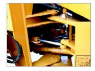
1. Large maintenance space is preserved in the front frame and enough room under the cab. Converter, gearbox installed separately for the convenience of maintenance.
