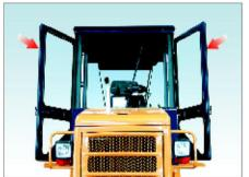
The cab can be opened from both side and could be reversed 180\* which means convenient for driver's work
